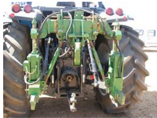
Figure 3: Three-point hitch dynamometer
