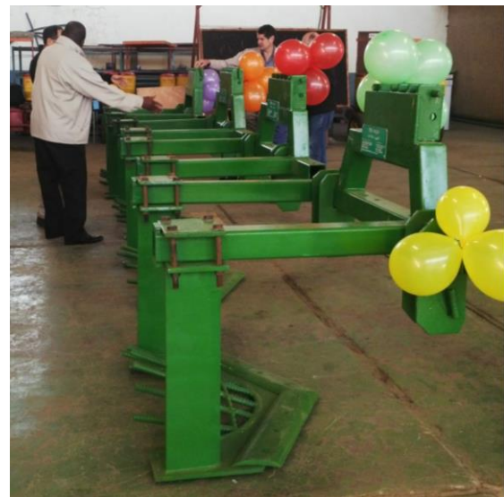
Figure 1: Cassava harvester according to the “dig and pull principle” being commissioned in South Africa
