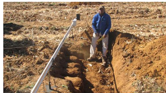
Figure 4: Soil profile measurement using the laser beam technology
