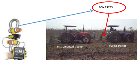
Figure 2: Implement draft determination by RON 2125S electronic dynamometer
